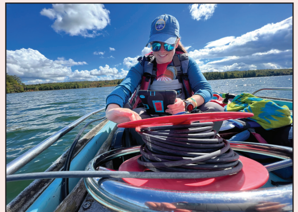
Lizzy Gallagher, 7 Lakes Alliance's assistant lake scientist, lowers a probe to measure water temperature and oxygen levels while collecting water samples in October. 7 Lakes Alliance collects and analyzes samples throughout the fall to determine when a lake's water "turns over" after being stratified by temperature throughout the summer.
