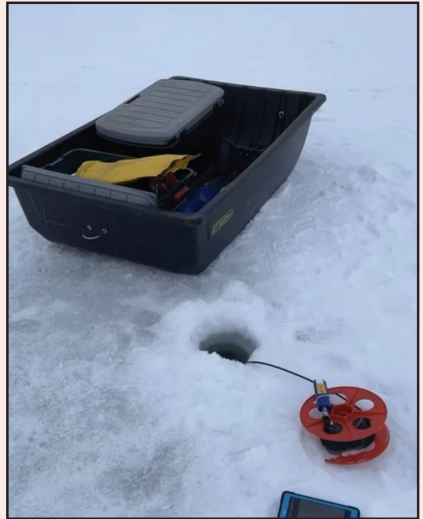
This probe records data beneath the ice, measuring characteristics such as temperature, dissolved oxygen, clarity, and other attributes.
