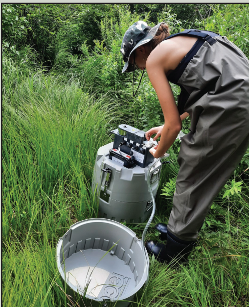
Colby Intern, Erin Coughlin, is setting up an autosampler on Great Meadow Stream.
