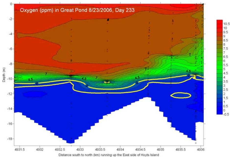
Oxygen contour along a south to north transect on Great Pond, 8/23/2006. Notice the slope of 7 ppm oxygen contour reaching up to a depth of 4 meters on the north end of the lake. This implies that >30% of the water at 4 meters was mixed upward from the hypolimnion.
