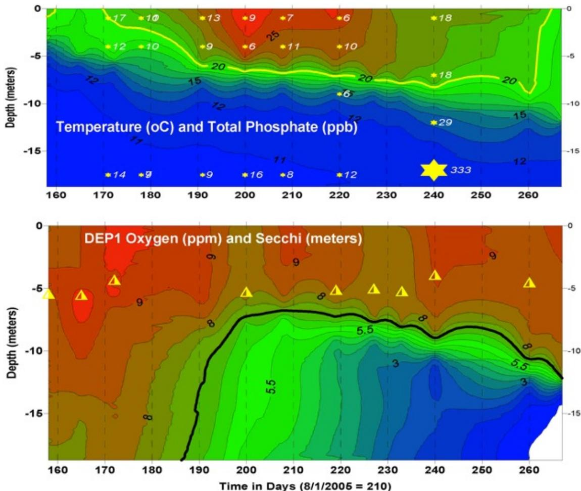
**Great Pond temperature and depth contours for 2005** (observation station DEP1 SE of Hoyt's island). Notice the thermocline formed at 10 meters depth and deep anoxia forming at day 230 in the hypolimnion (deep layer). Yellow triangles are Secchi depth and yellow stars are total phosphorus concentration. Notice the
